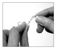
Push the end of the hearing aid hook firmly inside the new piece of tubing.
