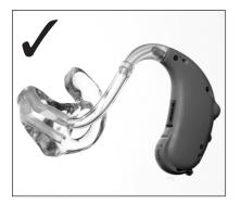
The mould should point away from the hearing aid as shown in the picture.
