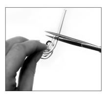
Use the old piece of tube as a measure for the new piece.
